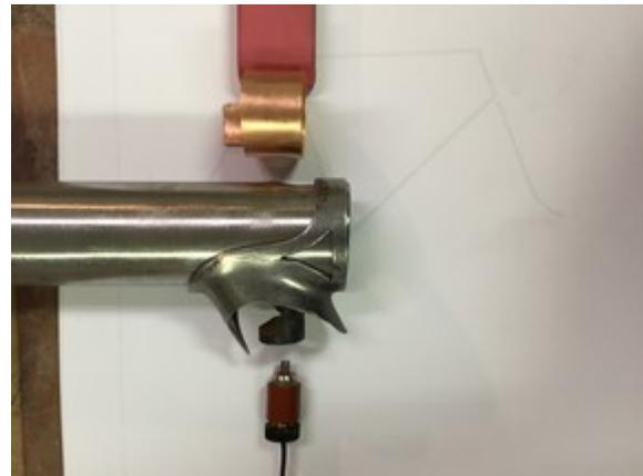
**Photos 5 & 6:** The partially reworked carbon brush and the finished brush, HT and slip ring laid out for visualization.
