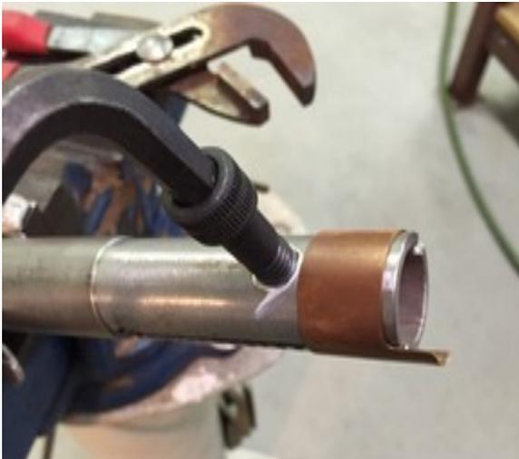
**Photo 16:** Slip ring on lug vise: Go very easy and in very small increments with every stretching step! Pliers compress the vise immediately to the left of the backed-off bolt in order to ease installation and removal of the slip ring.
