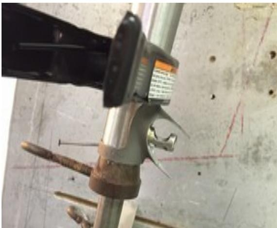
**Photo 9:** Checking the fit of the down lug, head tube and brush capsule receptacle prior to brazing.
