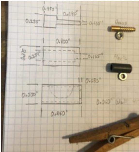
**Photo 7:** Dimensions of the brush, capsule and receptacle, from top to bottom.
