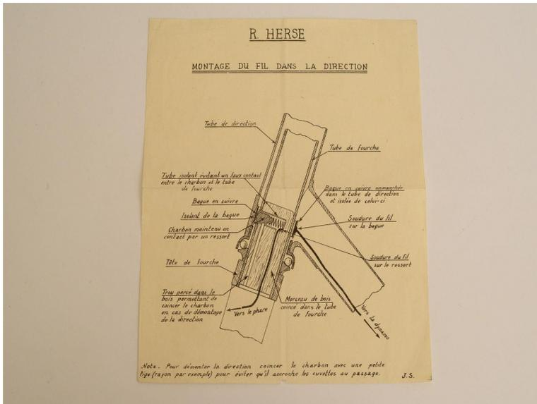
**Photo 1:** Drawing of the Herse slip-ring/carbon brush assembly
